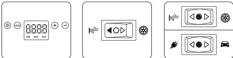
Press the "UNIT" to select the display unit. Then, press "-" or "+" to set the desired pressure. Press the mode switch to high-volume mode and inflation will start automatically and will automatically stop at a desired pressure level. When inflation is finished, turn both switches to OFF position.
