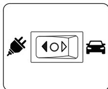
Plug the power cord into the AC socket in your house. For inflation, connect the high-volume hose to air pump's outlet, twist the hose to fix it. Before starting the deflation, connect high-volume hose to air pump's air inlet. Connect the high-volume nozzle to low pressure item. Use nozzels if needed. Press the power supply switch to house power supply mode.
