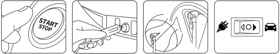
**STEP 2:** Press the "UNIT" to select the display unit. Then, press "-" or "+" to set the desired pressure. Press the mode switch to high-pressure mode and inflation will start automatically and will automatically stop at a desired pressure level. When inflation is finished, turn both switches (inflation mode switch and power supply mode switch) to OFF position.
