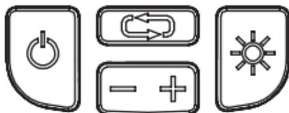
1. Long press (2 sec) the switch button "⏻" and the screen will turn on. If no operation is performed after switching the air compressor, it switch to hibernation mode in a 1.5 min.
