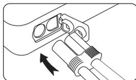
**STEP 1:** Open the silicone stopper of the product and insert the battery clamp into the corresponding hole of the product.
