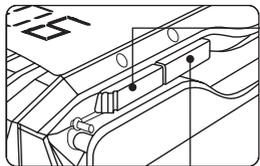
Press and hold the key for 3 seconds to turn on the flashlight, then the light button function changes from solid light to flashing, SOS distress signal light.
