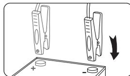
**STEP 2:** Connect the battery clamp to the positive and negative poles of the car battery (Red for the positive terminal and black for the negative terminal).
