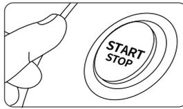
**STEP 3:** Start the engine. Do not cycle the jump starter for more than 3 seconds, pause for 1 minute between jump start attempts. This is necessary to let the jump starter battery cool down.
