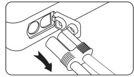
**STEP 4:** The plug is withdrawn from the jump starter first, and then the battery clips are removed from the positive and negative terminals.
