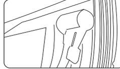
Connect one end of the inflation cable to the tire
