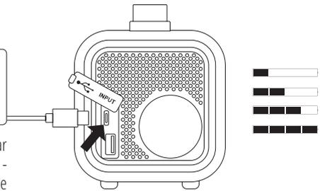
**NOTE:** Battery indicators show the current battery level (1 bar means under 25% of battery level, 2 bars - 25-50%, 3 bars - 50-75%, 4 bars 75-100%). Battery indicators will illuminate circularly while charging process and when all 4 indicators will be off - it means the charging process is finished.
