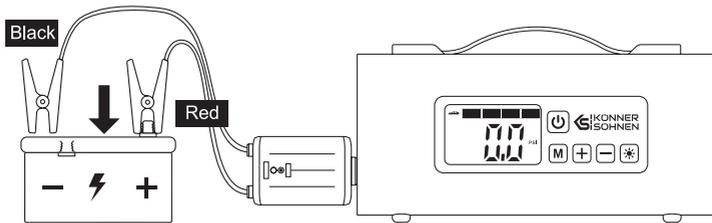
**Troubleshooting:** If smart battery clamps are illuminated with flashing red - polarities are reverse. Reverse the clamps to correct position.
