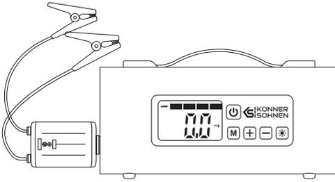
**STEP 1** – First insert smart battery clamps into the port of jump starter. If it is inserted completely, red indicator will flash on a jump starter cables. It means air compressor is discharged.
