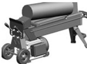
Release both operating handles so that the log pusher is fully retracted. Insert a triangular wedge of wood under the log and activate the log pusher to push the wedge under the jammed log. Repeat this process using progressively larger wedges until the jammed log is freed.
