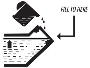
**Recommended motor oil:** SAE 10W30, SAE 10W40.
